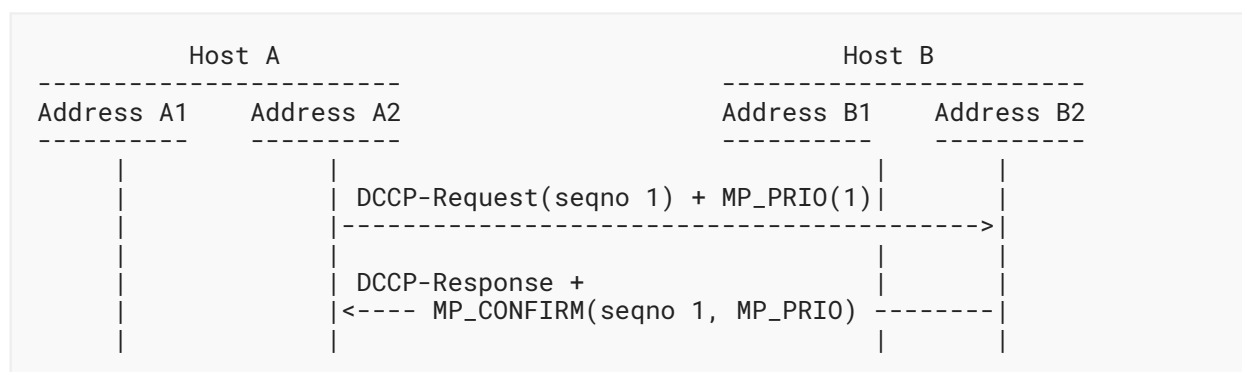
Figure 7: Example MP_CONFIRM Procedure
